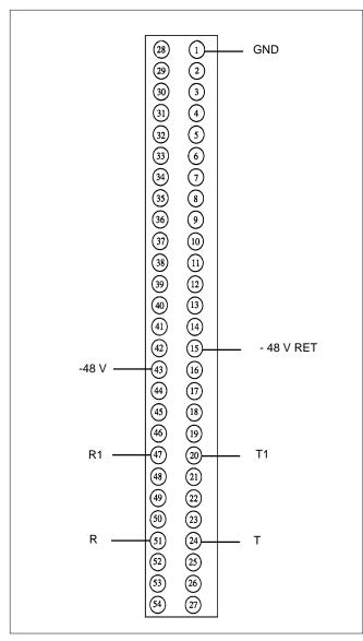
FIGURE 3. Connector Pin Assignments
